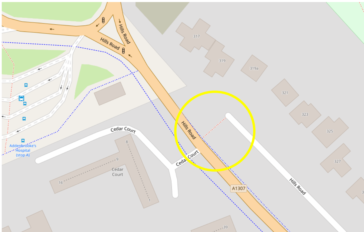
Figure 4: Potential cycle/footway link to divert some cycle traffic off the Hills Rd footway
